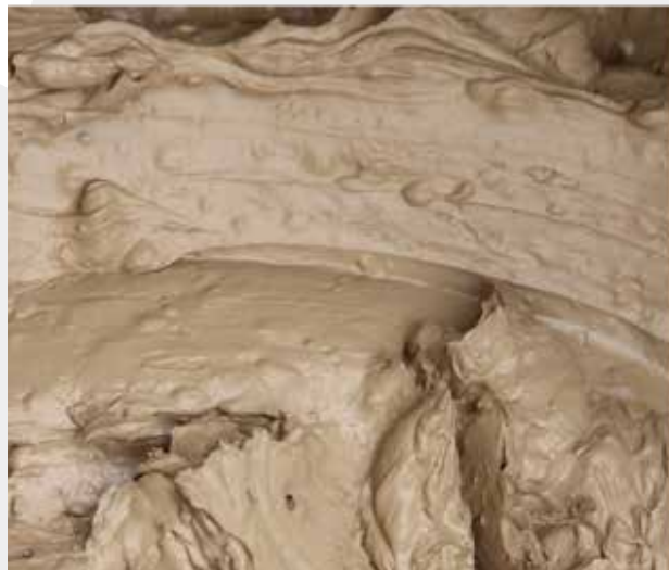
Clay mud produced through the washing process of sand and gravels.
